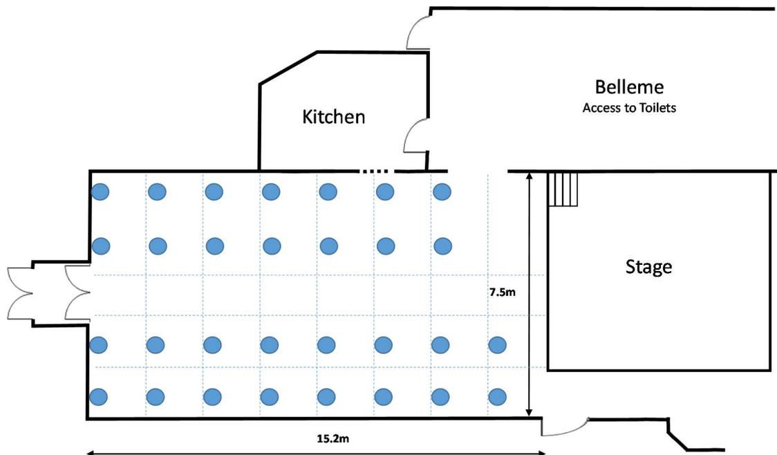
Figure 1 - GVH Main Hall capacity with 2m spacing
